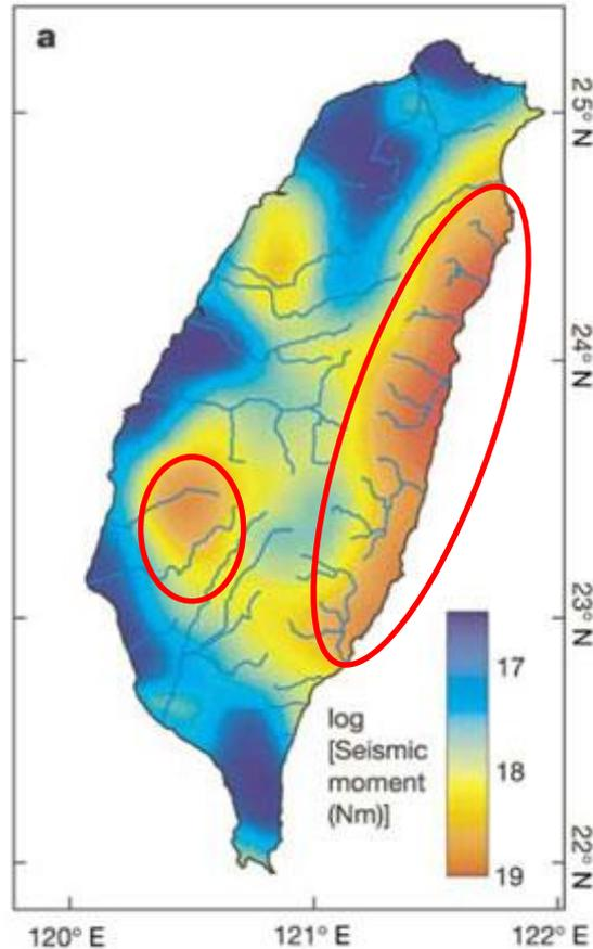
$$M_0 = \text{rigidity} \times \text{fault area} \times \text{fault slip}$$
